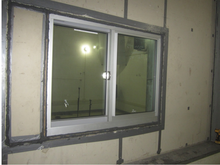
Receive Room View of Installed Specimen
