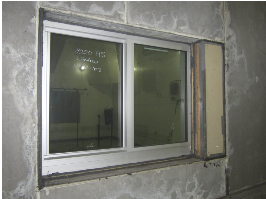
Source Room View of Installed Specimen
