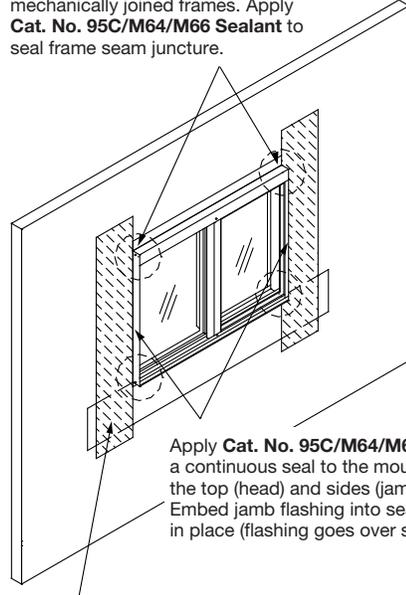
Apply **Cat. No. 95C/M64/M66 Sealant** as a continuous seal to the mounting flanges at the top (head) and sides (jamb) of window. Embed jamb flashing into sealant and fasten in place (flashing goes over sealant).
