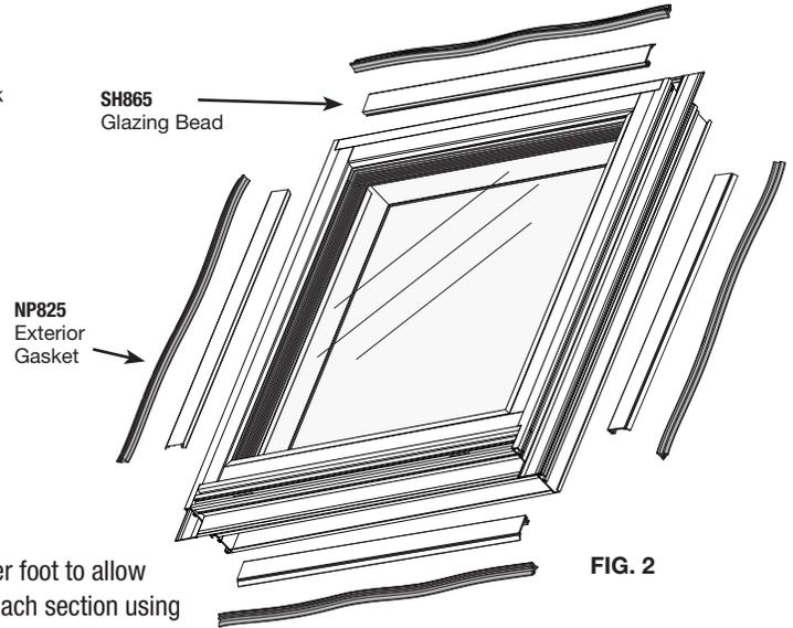
**Step 4:** Support the frame at a 10°-15° angle and insert the Glass Panel, working it into position against the frame blocks **Figure 2**
