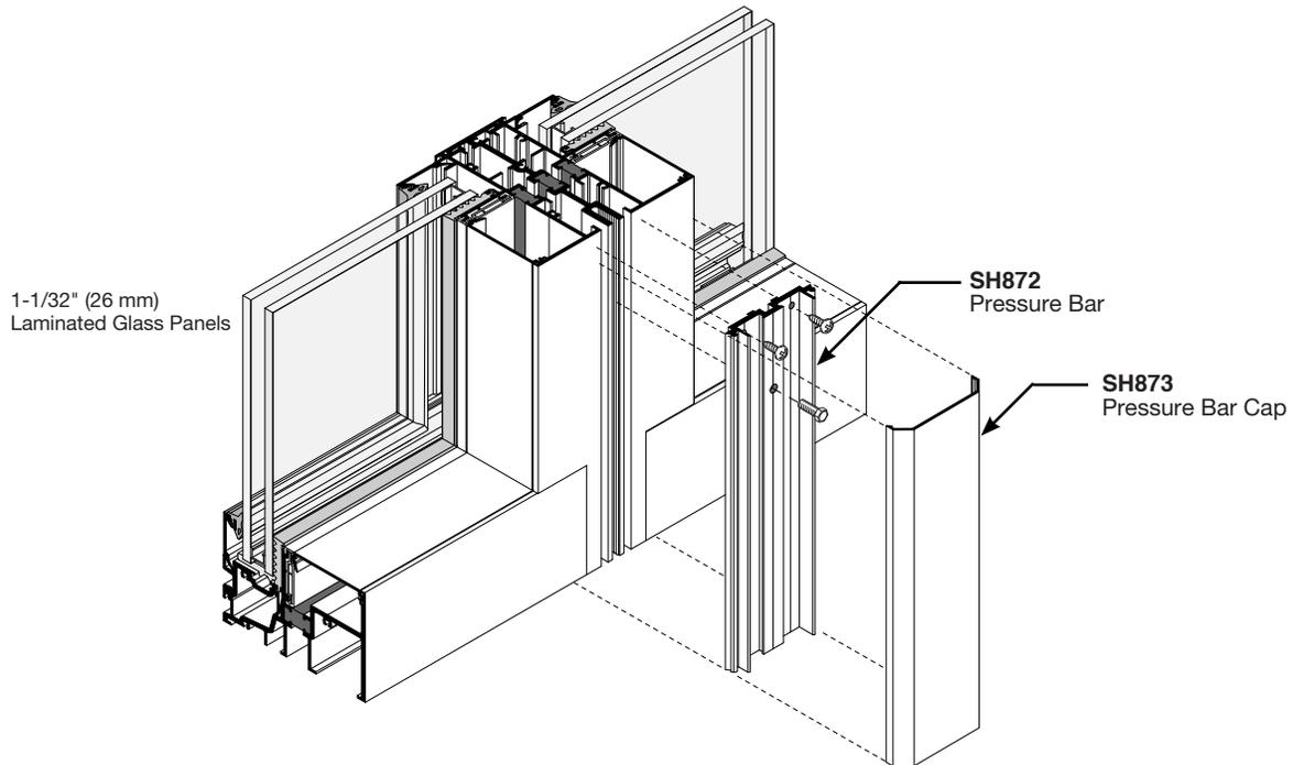
15. Center Pressure Bar vertically on exposed window jambs. Attach Pressure Bar to Mullion with a 1/4-20 X 1" HWH Screw. Spacing to be from shop drawing.
