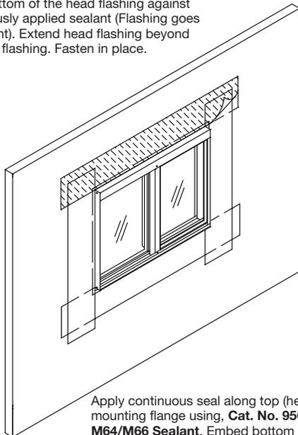
Apply continuous seal along top (head) mounting flange using **Cat. No. 95C/M64/M66 Sealant**. Embed bottom of head flashing against sealant (flashing goes over sealant). Extend head flashing beyond each jamb flashing. Fasten in place.
