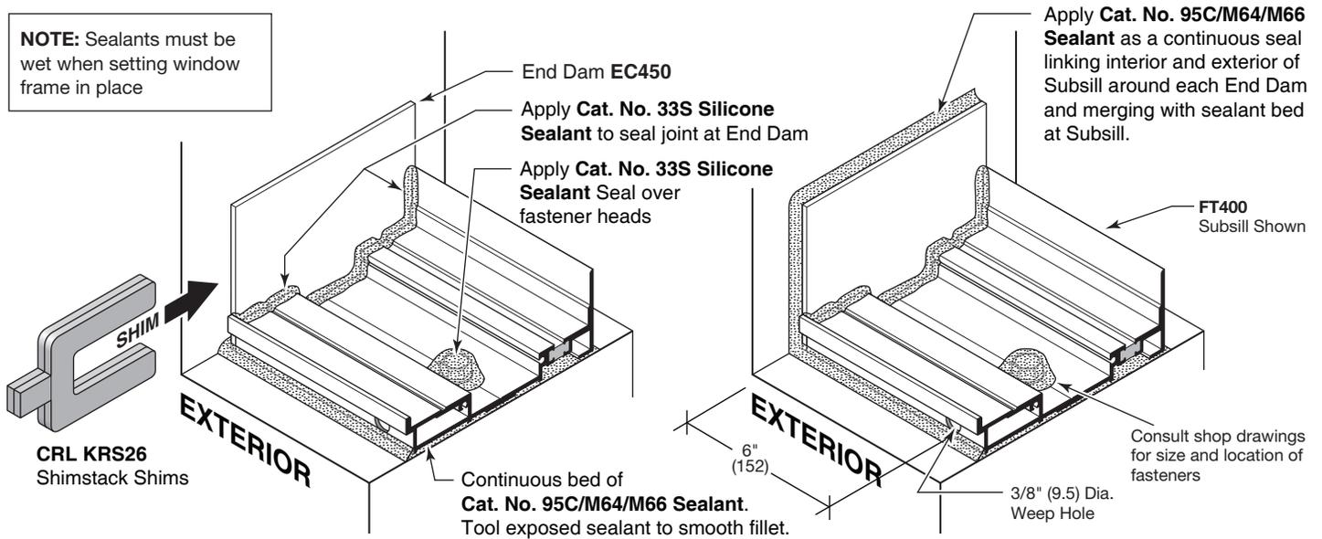
**NOTE:** If extruded Subsill is not used, it is recommended that a pan flashing be used. Pan flashing design and installation method is not determined by or warranted by U.S. Aluminum. Refer to approved project shop drawings for scope and intent of pan flashing requirements.
