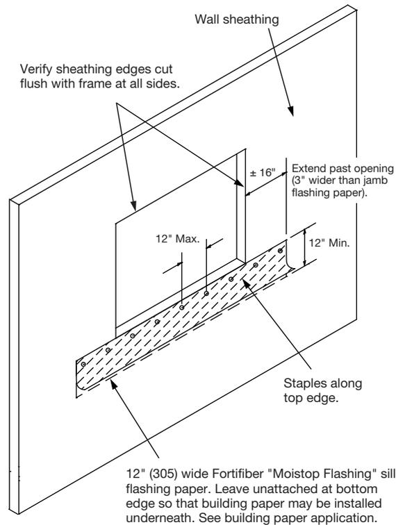
**NOTE:** Corrosion-resistant staples may be stainless steel or copper with 3/8" (9.5) leg for window flashing.
