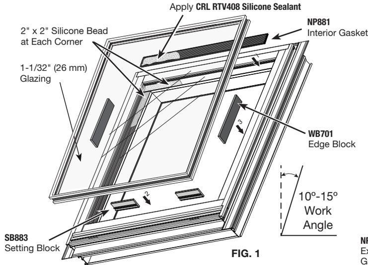
**Step 1:** Cut the Interior Glazing Gasket (supplied) to size and insert around the perimeter, sealing all end joints.
