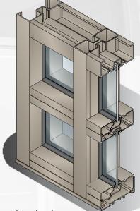
Fabrication and installation labor costs have always been a decisive factor in selecting framing systems for storefront projects. United States Aluminum offers cost efficient versatile Center Glazed Systems with clean lines and superb performance. All series may be interior or exterior glazed. A top load E.P.D.M. gasket is used to position and weatherseal the glass in the aluminum pocket. Center Glazed Systems are compatible with most United States Aluminum Entrance Doors.
