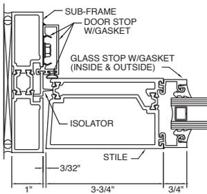
**HINGE STILE WITH 2" FRAME AND BUTT HINGE**
