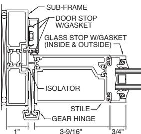
**HINGE STILE WITH 2" FRAME AND GEARED HINGE**
