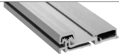
These U.S. Aluminum Full Surface Continuous Hinges have load bearing blocks every 5-1/8" (130) on the Standard Duty Hinge, and every 2-9/16" (65) on the Heavy-Duty Hinge. They are available in satin anodized and dark bronze anodized finishes, and stocked in 83" (2.11 m) lengths. A pack of installation screws is included with each Hinge. Replacement Screw Packs are also available separately.
