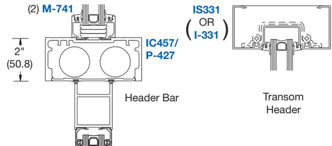
**NOTE:** Frame packages include TH400 threshold and transom sash with glazing gaskets for transom frames. When ordering frame for single door, specify handing. Visit [usalum.com](http://usalum.com) for additional information.
