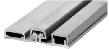
These U.S. Aluminum Full Surface Continuous Hinges have load bearing blocks every 5-1/8" (130.2) on the Standard Duty Hinge, and every 2-9/16" (65.1) on the Heavy-Duty Hinge. They are available in satin anodized and dark bronze anodized finishes, and stocked in 83" (2.11 m) lengths. A pack of installation screws is included with each Hinge. Replacement Screw Packs are also available separately.
