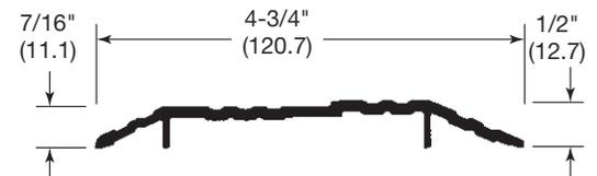
4-3/4" (120.7) THRESHOLD PREPARED FOR OFFSET PIVOT DOORS
