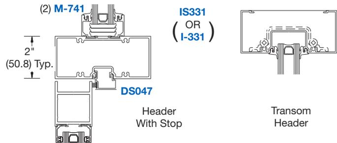
**NOTE:** Frame packages include TH250 threshold and transom sash with glazing gaskets for transom frames. When ordering frame for single door, specify handing. Visit [usalum.com](http://usalum.com) for additional information.
