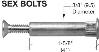
Used for securing push bars, surface mounted door closers, and other fixtures to 1-3/4" (44.5) doors. Knurled barrel fits a 3/8" (9.5) diameter hole. Available in aluminum and bronze finishes. Four bolts per package.
