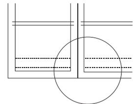
Allows existing doors to meet California Title 24 Handicap Code requirements of a 10" (254) bottom rail. Easily mounts between door stiles with double face tape. 6-3/4" (171) wide x 31-3/4" (806) long to fit 36" (914) doors. Other sizes available on request. One per package.
