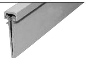
These U.S. Aluminum Concealed Leaf Continuous Hinges have load bearing blocks every 5-1/8" (130.2) on the Standard Duty Hinge, and every 2-9/16" (65.1) on the Heavy-Duty Hinge. They are available in satin anodized and dark bronze anodized finishes, and stocked in 83" (2.11 m) lengths. A pack of installation screws is included with each Hinge. Replacement Screw Packs are also available separately.
