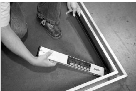
Unfold locator arm.
