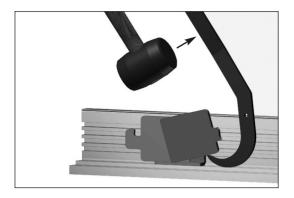
STEP 2: Using a rubber or plastic mallet, apply firm blows to the upper handle of the Extractor to break any seal that may have formed between the glass taper and the base shoe due to weathering. If you feel movement, stop and relocate the Extractor further under the taper and repeat the process. The goal is to raise the taper corner about one inch (see illustration below).
