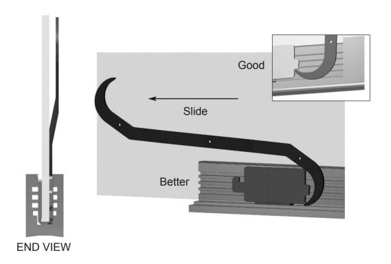
Position the tool as illustrated above and slide to the left while holding with both hands. Try to wedge the tip of the Extractor under the main part of the taper body rather than the ear. Depending upon the type of tapers used and the size of the base shoe, the bottom gap will vary. If you cannot get the tool under the bottom edge of the taper then the ear protrusion will be adequate.
