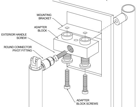
2.A. FOR GLASS MOUNT HANDLE. Remove Socket Head Cap Screw from Interior Pivot Bracket and Exterior Bracket. Be careful not to lose Gaskets located between Interior and Exterior Brackets
