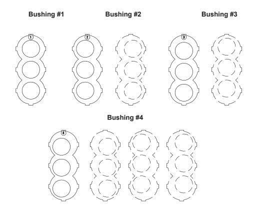
Use Bushing #4 when the "Hole Centers" and the 4-1/8" dimension from door's edge are both off 1/16" in either direction.
