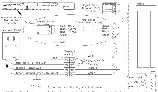
Wall Mount Transformer or other Power Supply (1). The most common output is 24 Volts AC or DC (regulated or linear). Use a Class II isolated supply for safety (UL listed or recognized).
