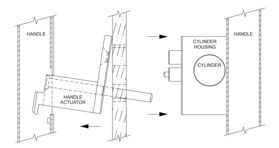
4. Loosen set screw holding cylinder in place with an Allen wrench.
