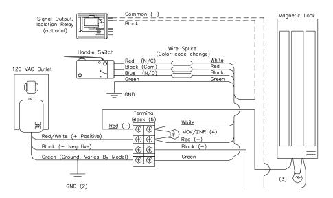
Dry Contact Switch Input to the Magnetic Lock Controller
