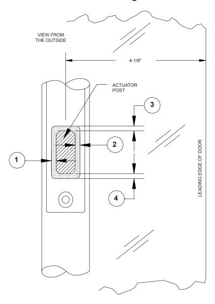
To insure proper handle operation the Actuator Post must be centered within the rectangular slot in the handle. View the Actuator Post where it enters the rectangular slot in the handle, through the door glass. With the handle dogged in the operational position, dimension "1" should be smaller than dimension "2". Dimension "3" and "4" should be equal. With the handle dogged in the unlocked position, dimension "2" should be smaller than dimension "1". Dimension "3" and "4" should be equal.
