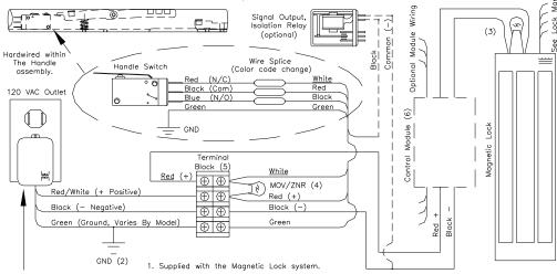
Wall Mount Transformer or other Power Supply (1). The most common output is 24 Volts AC or DC (regulated or linear). Use a Class II isolated supply for safety (UL listed or recognized).
