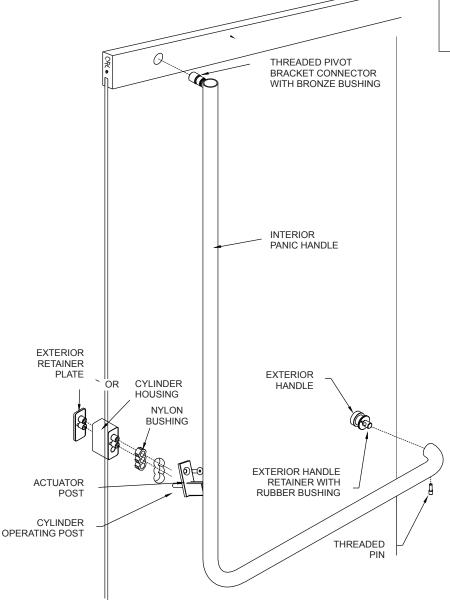
Apply THREADLOCKER to all fasteners used to mount handle on doors.
