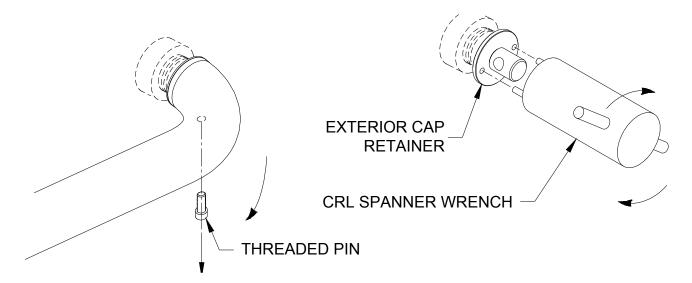
4. Unscrew the retainer caps holding the exterior horizontal handle to the plywood, being careful that the handle does not fall from the backside of the plywood. Remove rubber bushing for re-use during installation to the door. →
