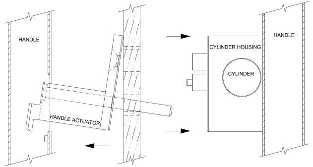
Loosen set screw holding cylinder in place with an Allen wrench.
