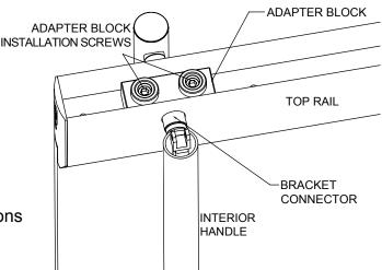
4.A. GLASS MOUNT HANDLE. Insert rubber bushing into glass hole at the top and the bottom of glass door. Place exterior pivot bracket against exterior side into notched portion of glass. Align interior handle with exterior pivot bracket and tighten low head cap screw.
