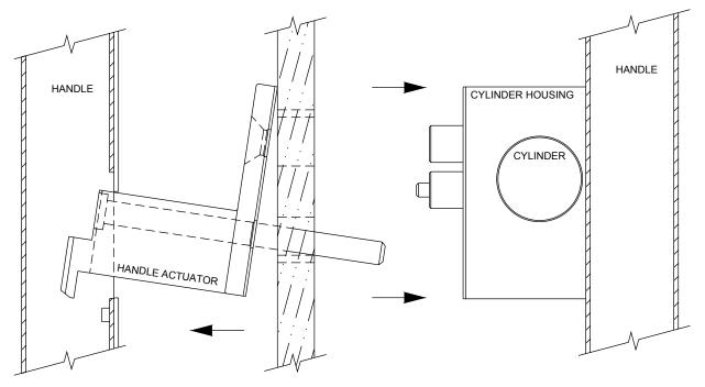
Loosen set screw holding cylinder in place with an Allen wrench.
