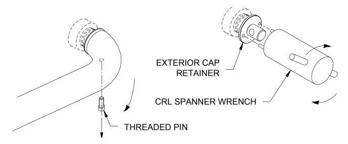
Unscrew the retainer cap holding the exterior horizontal handle to the plywood, being careful that the handle does not fall from the backside of the plywood. Remove rubber bushing for re-use during installation to the door. →
