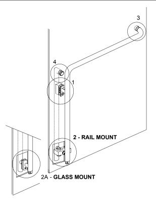
actuator post tilt the actuator post toward the horizontal handle section, then remove. Be careful not to lose the cylinder-operating pin, handle return plunger and spring, or the triple hole bushing.  $\Psi$
