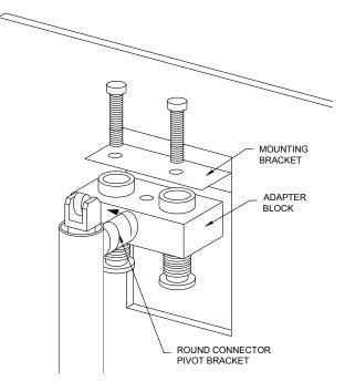
2.A. FOR GLASS MOUNT HANDLE. Remove Socket Head Cap Screw from Interior Pivot Bracket and Exterior Bracket. Be careful not to lose Gaskets located between Interior and Exterior Brackets. →
