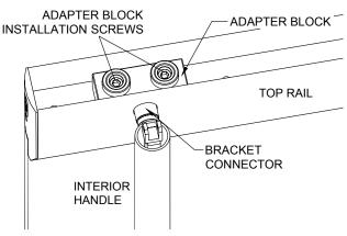
CRL Door Rails installation instructions for possible adjustments of the top rail.
