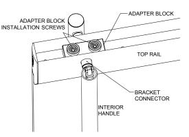
Install the Adapter Block into the Bottom Rail. Insert the handle fitting into the Adapter Block and tighten the setscrew.
