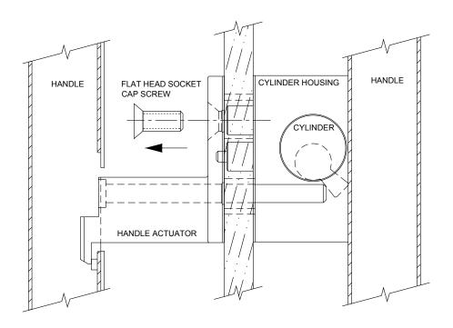
3. Pull handle away from glass. Remove handle actuator from handle.
