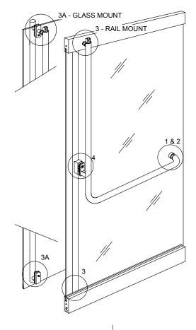
1. Push exterior horizontal handle retainer with rubber bushing through glass hole from interior side, into horizontal handle, and tighten with spanner wrench.
