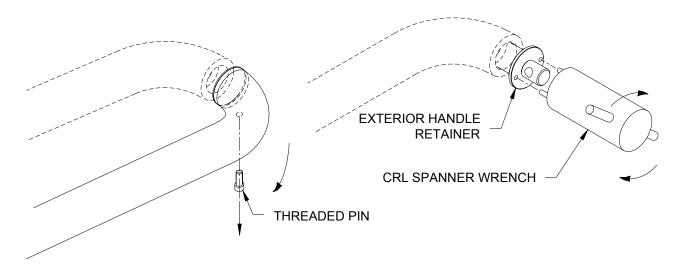
4. Unscrew the retainer cap holding the exterior horizontal handle to the plywood, being careful that the handle does not fall from the backside of the plywood. Remove rubber bushing for re-use during installation to the door. →
