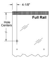
Use Bushing #1 when the "Hole Centers" dimension is correct and the 4 1/8" dimension from door's edge is accurate.
