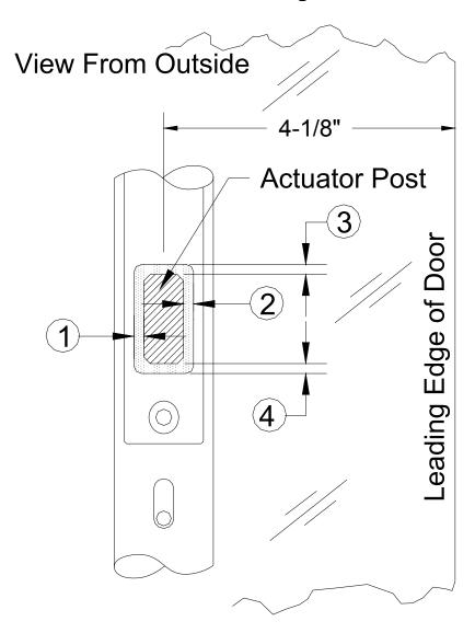
To ensure proper handle operation the Actuator Post must be centered within the rectangular slot in the handle.
