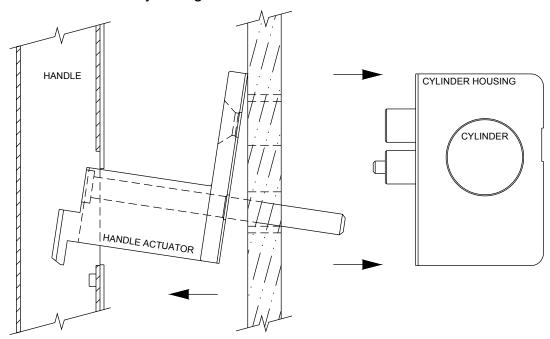
4. Loosen set screw holding cylinder in place with an Allen wrench.
