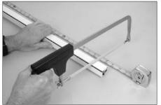
Diagram 7 - Cutting Top and Bottom Rails
