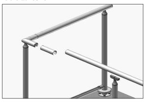
**4b.** Surfaces to be bonded should be cleaned with Cat. No. MEK1GL Solvent. Please follow the bonding instructions on the Cat. No. 32629 Adhesive and Cat. No. 7075 Activator packaging.
