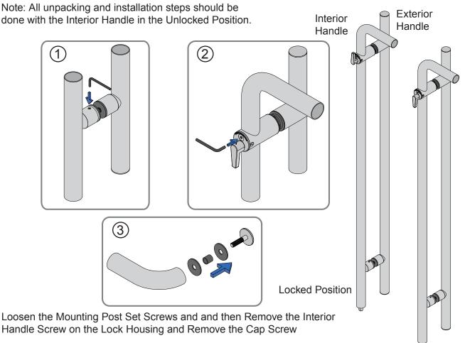
Separate handles, remove parts and store in a safe place for later use.
