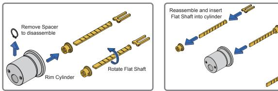
4. Install the Adaptor onto the new Rim Cylinder and reattach the new base and Cylinder to the Exterior Handle.
