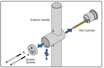
3. Disassemble the new Rim Cylinder to rotate the Flat Shaft to vertical position and reassemble.
