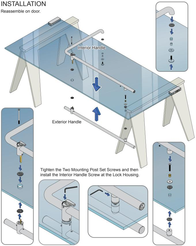
All LLPA and DLLPA Handles come with SFIC Rim Cylinder and Core that can be replaced with either SFIC or LFIC Rim Cylinders and Cores.
