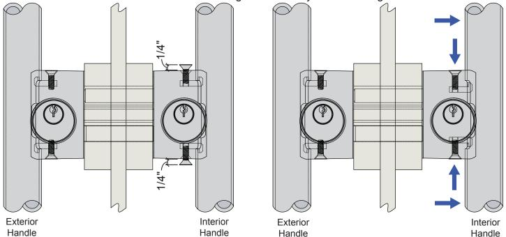
3. Remove the 2 cap screws from the inside of the Cylinder Housing, and remove the housing from the board. Remove the exterior handle, rubber bushings and save it for re-use during installation to the door.
