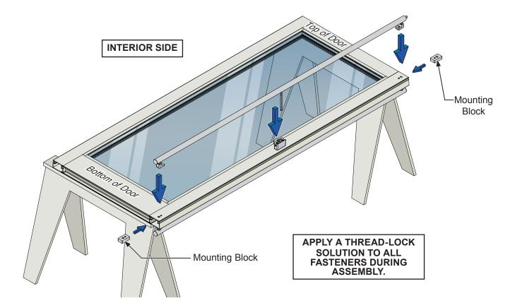
10. Hold the mounting blocks in place and attach the handle to the door using the two 5/16-18 x 1" low head socket cap screws.
