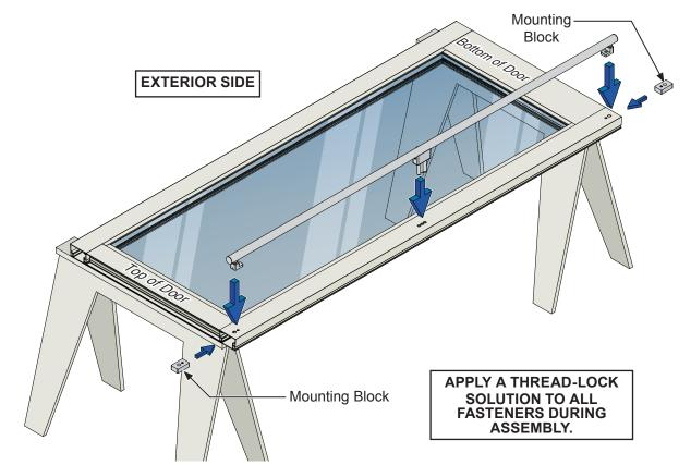
6. Hold the mounting blocks in place and attach the handle to the door using the two 5/16-18 x 1" low head socket cap screws. (Fig. 9)
