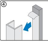
Remove backing and install rubber insert.
