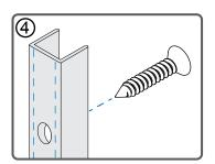
Secure using fasteners appropriate for the surrounding substrate. Fasteners not included.
