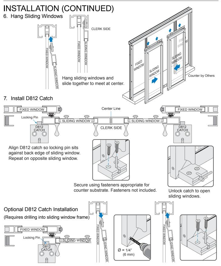
Remove windows to drill 1/4" (6 mm) hole in bottom corner. Hang windows and align D812 catch so locking pin engages. Secure using fasteners appropriate for counter substrate. Fasteners not included.
