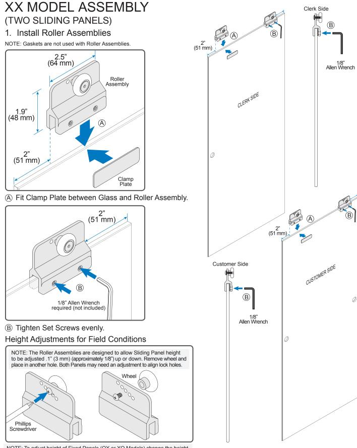
NOTE: To adjust height of Fixed Panels (OX or XO Models) change the height and/or quantity of Setting Blocks installed in Bottom Rail.
