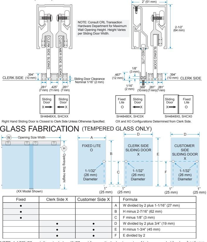
NOTE: 1-1/32" (26 mm) diameter holes, 1" (25 mm) from vertical edge to center of hole are needed for door hardware.
