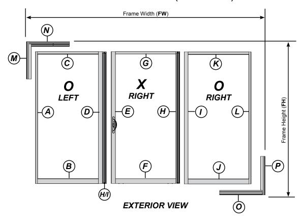
Your order has been carefully fabricated, inspected, and packaged to work order specifications. We have placed an Indicator Label on the inside or back side of each part before final packaging. Use the Identification Key (above) to organize and lay out each Series 3000 Sliding Patio Door System before proceeding with the assembly process.
