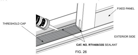
4. Seal the interior side of the fixed panel to the frame using Cat. No. RTV408 or Cat. No. 33S sealant. Run a continuous bead of sealant at the sill, jamb, and head. (FIG. 27)
