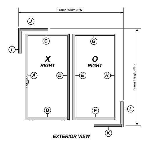
Your order has been carefully fabricated, inspected, and packaged to work order specifications. We have placed an Indicator Label on the inside or back side of each part before final packaging. Use the Identification Key (above) to organize and lay out each Series 3000 Sliding Patio Door System before proceeding with the assembly process.
