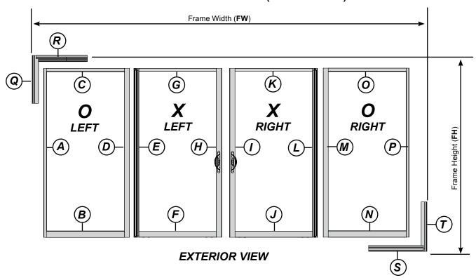
Your order has been carefully fabricated, inspected, and packaged to work order specifications. We have placed an Indicator Label on the inside or back side of each part before final packaging. Use the Identification Key (above) to organize and lay out each Series 3000 Sliding Patio Door System before proceeding with the assembly process.
