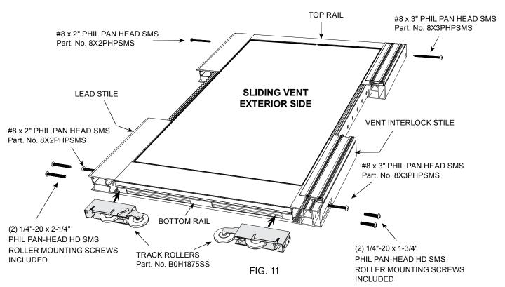
12. Complete the glazing and assembly of all sliding and fixed vents. Adjust rollers to their fully retracted position before installing doors.
