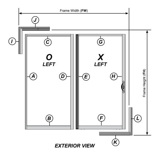
Your order has been carefully fabricated, inspected, and packaged to work order specifications. We have placed an Indicator Label on the inside or back side of each part before final packaging. Use the Identification Key (above) to organize and lay out each Series 3000 Sliding Patio Door System before proceeding with the assembly process.
