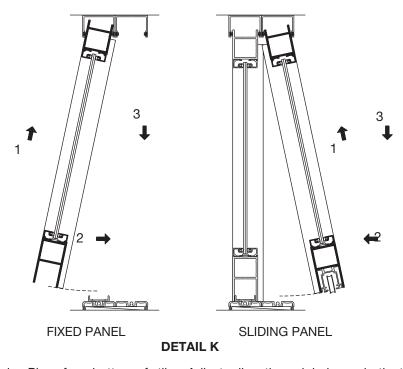
Remove SP23733 Nylon Plugs from bottom of stiles. Adjust rollers through holes on both stiles to align panels and ensure proper engagement of hookbolt lock. Turn adjusting screws clockwise to raise panel and counterclockwise to lower it. See DETAIL L. Reinstall SP23733 plugs.
