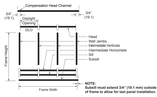
3. Position DJ456 Drill Jig on end of each member and drill holes for assembly screws. Use #7 bit to drill .201" (5.1 mm) holes. Refer to shop drawings for hole locations
