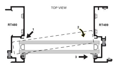
Install glass panel into frame by first angling the panel into the deep pocket. Swing the other end around and into the shallow pocket. Lower the panel down onto the setting blocks.
