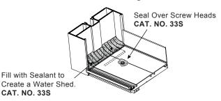
**NOTE:** Not for use near insulating glass units with butyl sealant.
