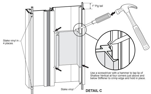
5. Insert the VS200 vinyl into the RT489 mullion and leave a 1" pig tail at each end and stake in place.
