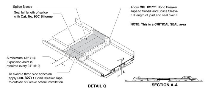
3. If there are no entrances, start installation at wall jamb unit. Apply silicone to end dam contact area. **See DETAIL R**. Set first panel inside subsill and in place.
