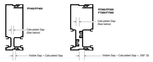
Expansion Mullions must be used to accommodate thermal movement in long run elevations.
