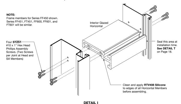
2. After panels are assembled, apply a bead of **RTV408 Silicone** to joint between verticals and sill members, from the underside, to ensure a watertight installation. **See DETAIL J**.
