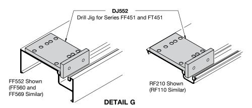
Drill .201" (5) Holes using a Cat. No. 80107 #7 Drill as Shown
