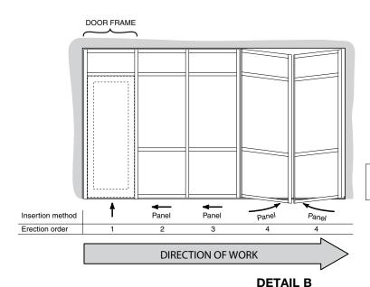
Units are inserted into an opening from LEFT to RIGHT
