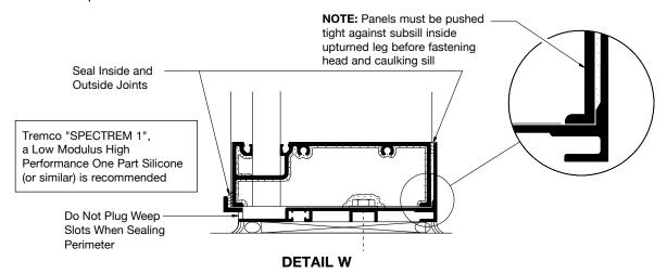
6. When interior glazing a multistory building, exterior perimeter sealing must be done before glazing, unless caulking is to be done from the exterior as a secondary operation.
