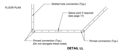
It is recommended that elevations with corners at both ends have at least one expansion member to allow for minor adjustments.
