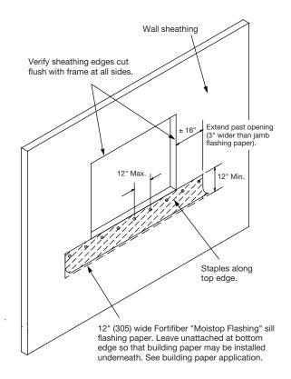
**NOTE:** Corrosion-resistant staples may be stainless steel or copper with 3/8" (9.5) leg for window flashing.
