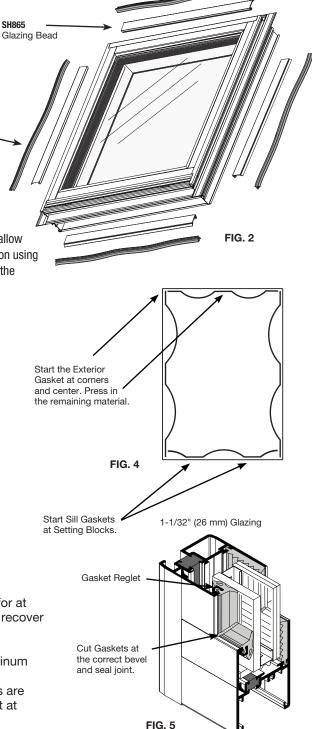
Step 1: Cut the Interior Glazing Gasket (supplied) to size and insert around the perimeter, sealing all end joints.
