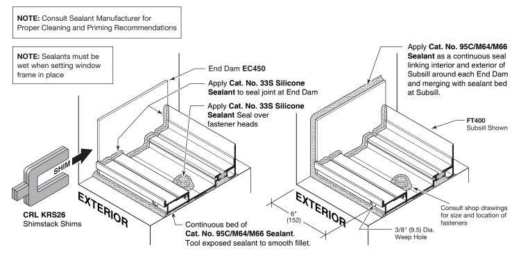
**NOTE:** If extruded Subsill is not used, it is recommended that a pan flashing be used. Pan flashing design and installation method is not determined by or warranted by U.S. Aluminum. Refer to approved project shop drawings for scope and intent of pan flashing requirements.
