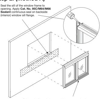
Shim and adjust window to achieve square, plumb, and level condition use corrosion resistant fasteners. Fasten within 10" and no closer than 5" in each direction from every corner. Secure window around frame opening with equivalent of five fasteners at 15" O.C. maximum.
