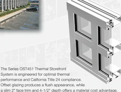
Additional features include injection molded water deflectors, a continuous head and sill, and a top-load EPDM gasket that permits interior or exterior glazing. The available OST451 SSG model provides uninterrupted horizontal glass spans for a streamlined aesthetic.
