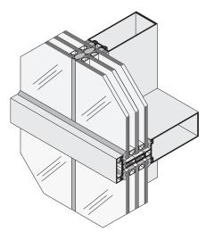
SERIES HP3253SG High Performance Structural Silicone Vertical Glazed Curtain Wall
