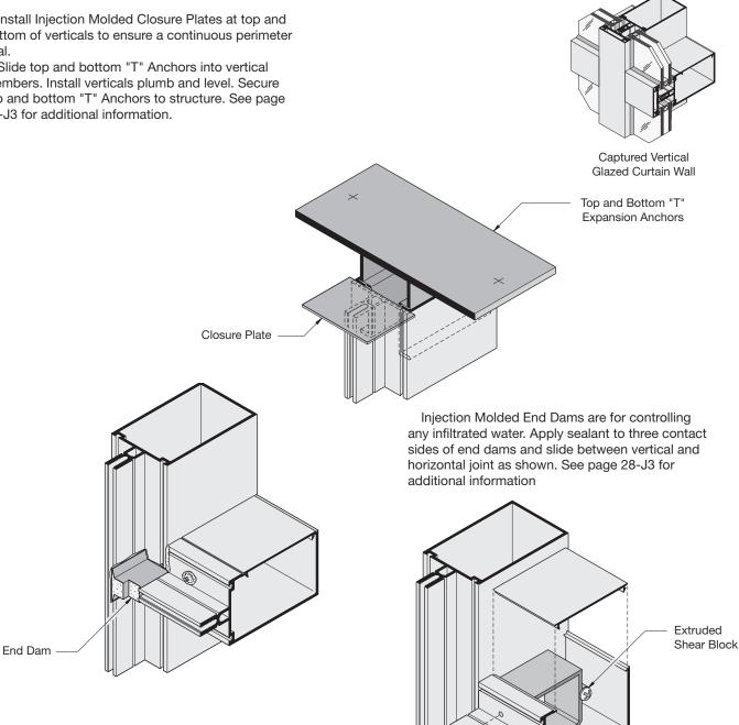
Extruded Aluminum Shear Blocks are furnished to ensure extra strong horizontal to vertical joinery. Attach shear blocks to verticals and horizontals to shear blocks with screws provided. See page 28-J3 for additional information.
