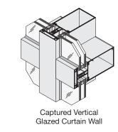
NOTE: Open Back Side of Top and Intermediate Horizontals are Shown. The Open Back is Down at the Bottom Horizontal Only.
