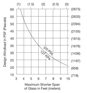
Stress on structural silicone should not exceed 20 PSI (137 KPa) for a 6:1 safety factor.
