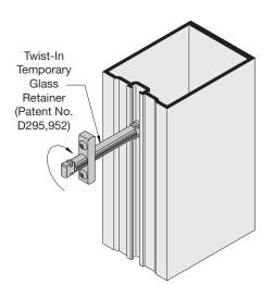
Reusable Twist-In Temporary Glass Retainers hold the glass in place during the structural silicone curing period. The plastic retainer is designed to work for both 1" (25) and 1/4" (6) infills.
