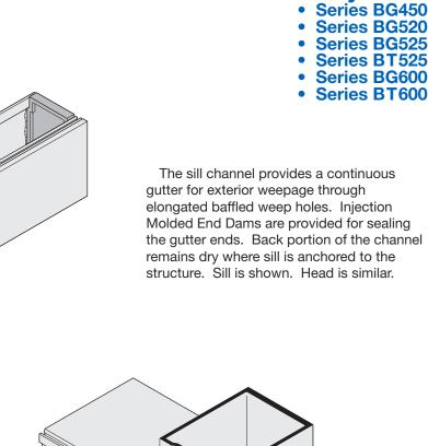
A uniquely designed Injection Molded Water Deflector is used for weeping infiltrated water to the exterior at the intersection of the intermediate horizontal and vertical mullions. The Contoured Water Deflector allows for an uninterrupted gasket seal at the intersection of intermediate horizontal and vertical mullions.
