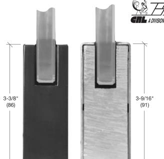
Typical Top or Bottom Rail for 150 and 250 Series Doors and Sidelites
