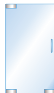
Single Door With Top and Bottom Pivots and a EUR205 Patch Lock
